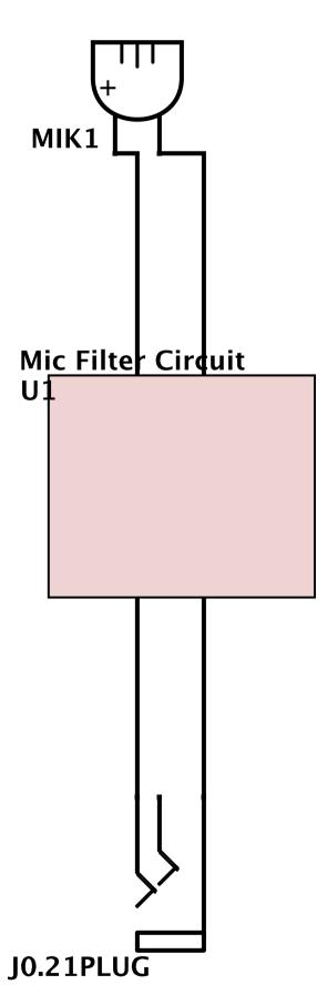
0.21inch Mic plug pinout: Tip: PTT (no wiring to MIC) Middle ring: Mic High
